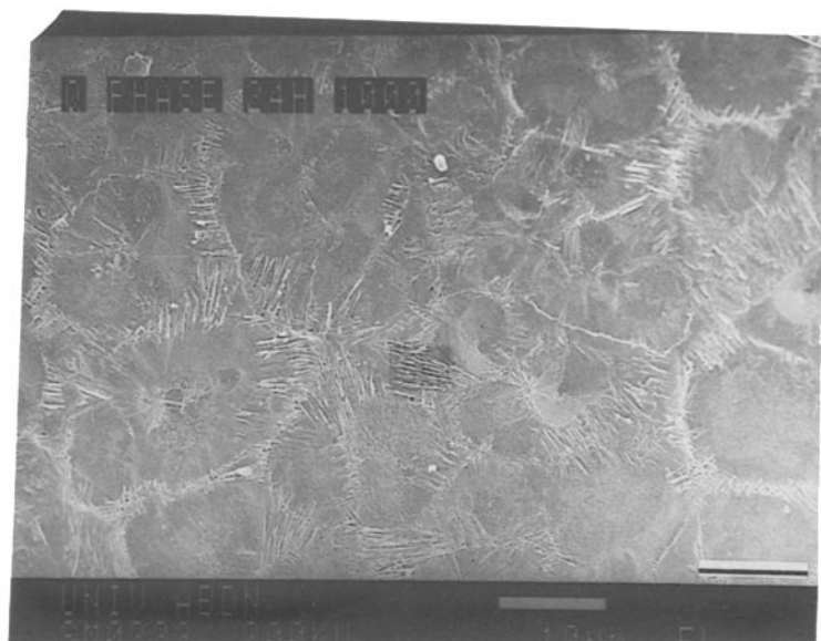
Figure 3 Scanning electron micrograph of a fractured surface of crystallized glass of composition (51.28 CaO, 7.70 MgO, 33.32 Al 2 O 3 , 7.70 SiO 2 (mol %)) heat treated for 24 h at 1000°C, which had been etched with HF (10 vol%) for 3 min. Scale bar = 10 μm.
