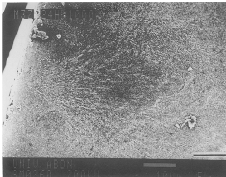
Figure 5 Scanning electron micrograph of a fractured surface of crystallized glass of composition (51.28 CaO, 3.85 MgO, 3.85 ZnO, 33.32 Al 2 O 3 , 7.70 SiO 2 (mol %)) heat treated for 24 h at 1000° C. Etching conditions identical to those mentioned in Fig. 3. Scale bar = 10 μm.
